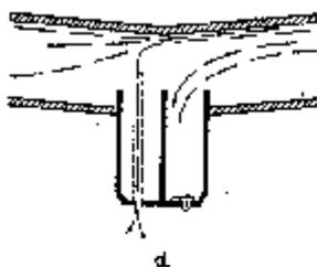
Next spray cycle. Water initially sprays through the brass tube on the left side. The heat from the liquid melts the ice plug blocking the right half of the nozzle and spraying resumes in the normal manner as shown in a.
