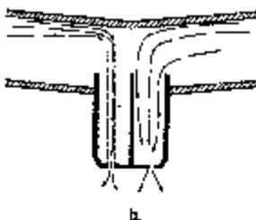
Draining. Brass tube in left half drains quickly, until liquid level is below its top. Then only right half continues to drain.
