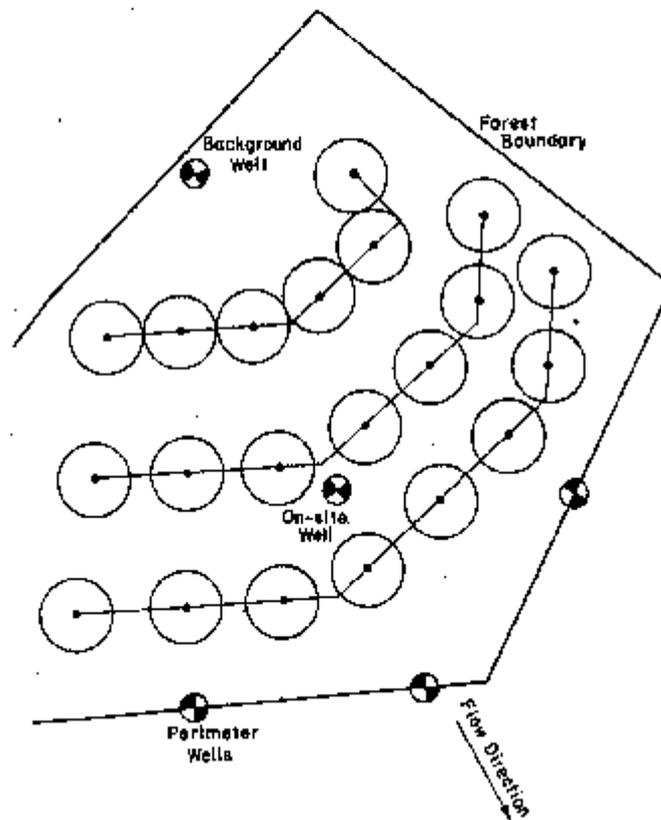
Figure 2-5. Typical monitoring layout.
