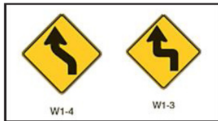
Two options for two sequential curves.
