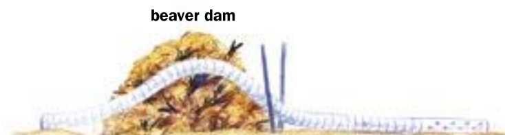
Figure 5-12. Massachusetts Beaver Pond Leveler
