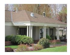
Excerpt from the FBC 308.3.1 Five or fewer persons receiving care. A facility such as the above with five or fewer persons receiving such care shall be classified as Group R-3 or shall comply with the Florida Building Code, Residential provided an automatic sprinkler system is installed in accordance with Section 903.3.1.3 or with Section P2904 of the Florida Building Code, Residential.
