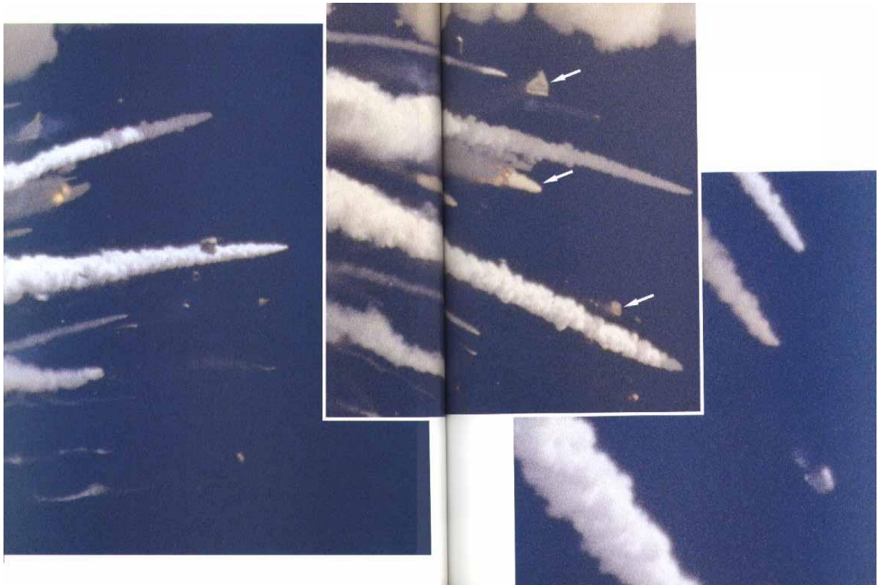
Fig. 16. Hurling out of the fireball at 78 seconds are the Orbiter's left wing (top arrow), the main engines (center arrow) and the forward fuselage (bottom arrow). In the photo below [bottom right], it plummets earthward, trailed by smoking fragments of Challenger.
