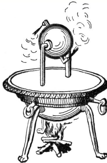
Aeolipile (Hero Engine)
