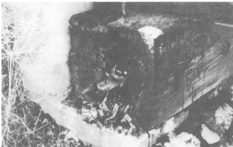
Figure 5-14. Advanced wood decay in crosstie.
