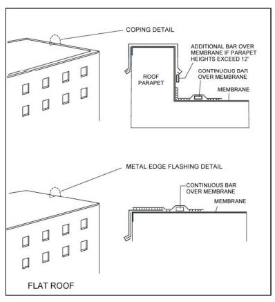
membrane (see detail figures) is an effective means of strengthening the attachment.
