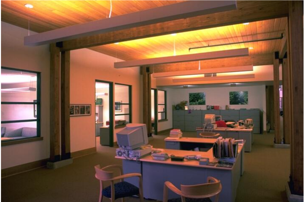
Figure 4 Minimize direct glare with indirect lighting.
