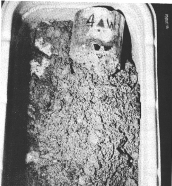
b. After freezing and thawing
