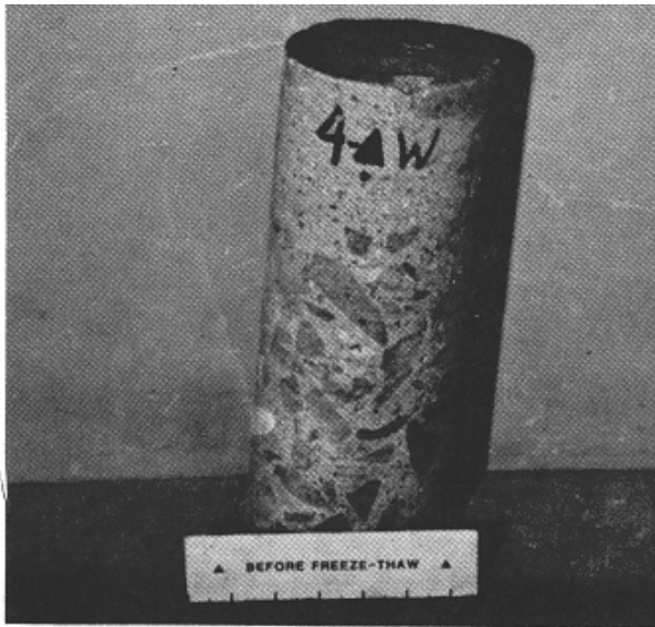
a. Before freezing and thawing
