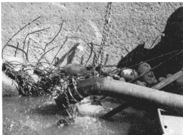
a. Debris collected behind wall baffle
